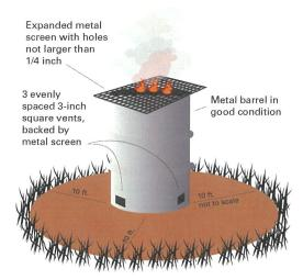
Ground cleared down to mineral soil or gravel at least 10 feet on each side of incinerator
