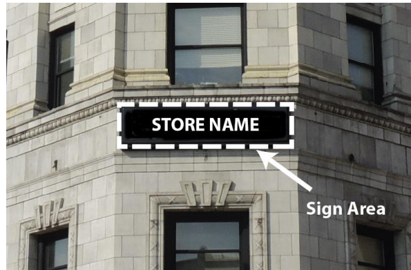
Figure O: Illustration of computing the sign area for wall signs with a background panel or cabinet.
